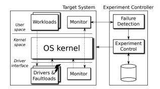
Fig. 1. System model and experiment setup
