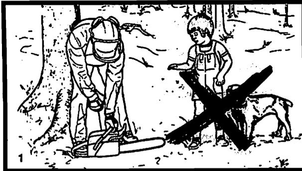
The use of any chain saw may be hazardous. The saw chain has large, sharp cutters. If the cutters contact your flesh, they will cut you, even if the chain is not moving. At full throttle, the chain speed can reach 45 mph (20 m/s). It is important that you read, fully understand and observe the following safety precautions and warnings. Read the owner's manual and the safety instructions periodically. Pay special attention to the section on reactive forces, pages 10 to 13.
